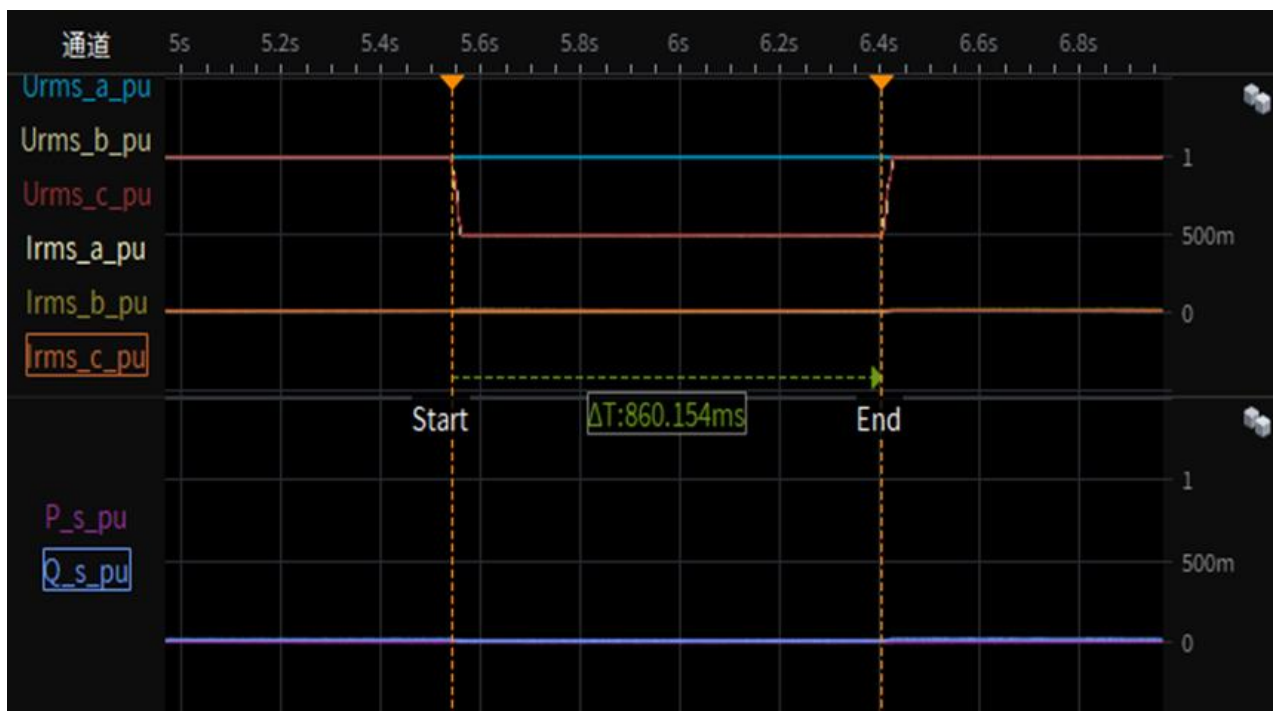
Test 6-Depth of fault phase: 0.5p.u., LV two-phase-asymmetrical (type D), 0% load Test overview(voltage,current,active and reactive power)
