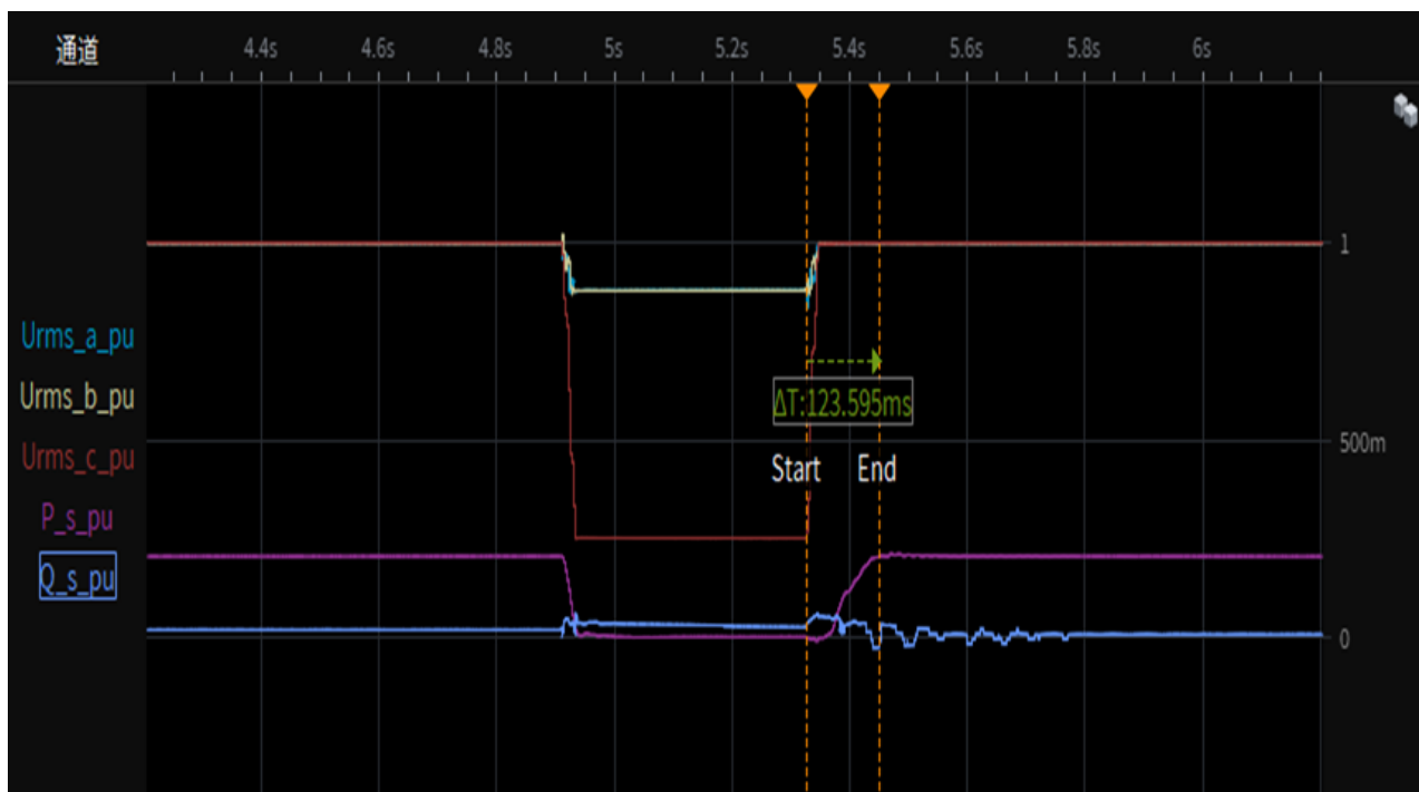
Test 2a-1.4 Depth of fault phase: 0.25p.u.,two-phase-asymmetrical (type D),20% load restoring time
