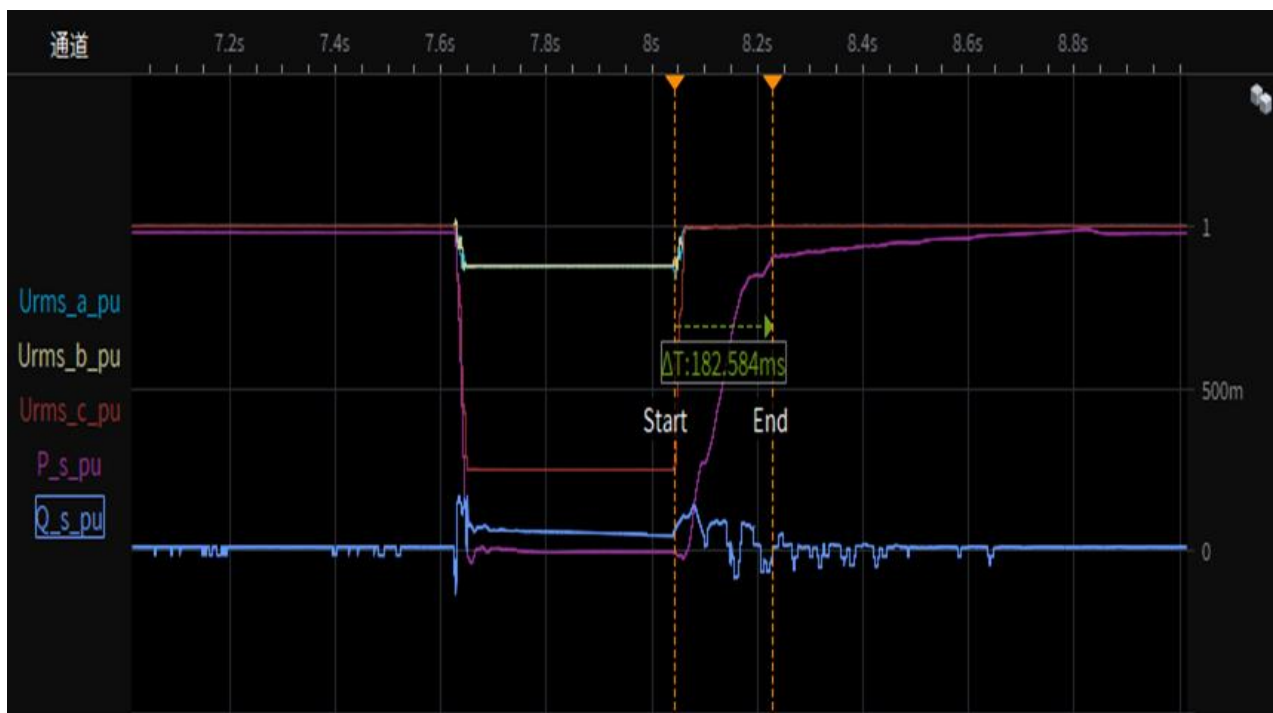
Test 2a-2.4 Depth of fault phase: 0.25p.u., two-phase-asymmetrical (type D), 95% load restoring time
