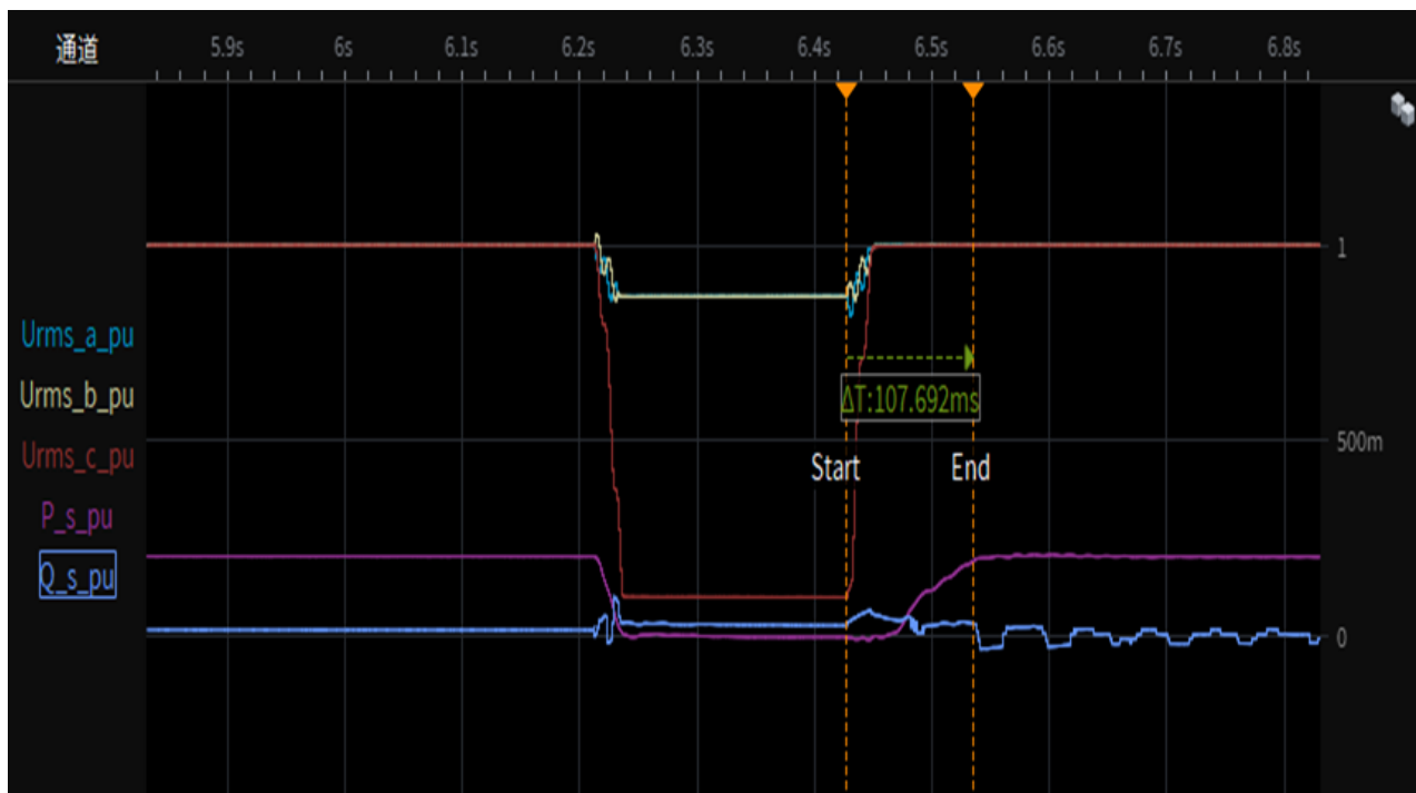
Test 1a-1.4 Depth of fault phase: 0.1p.u., two-phase-asymmetrical (type D),20% load restoring time
