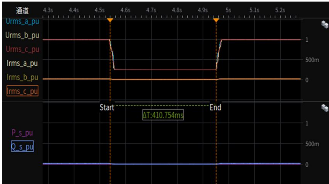
Test 2s-1.1 Depth of fault phase: 0.25p.u.,three-phase-symmetrical (type A),20% load Test overview(voltage,current,active and reactive power)
