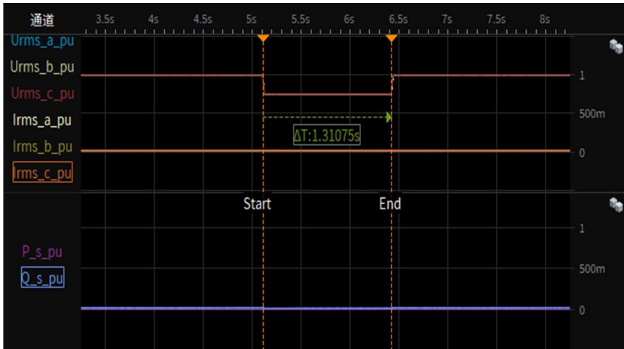
Test 4s-1.1 Depth of fault phase: 0.75p.u.,three-phase-symmetrical (type A),20% load Test overview(voltage,current,active and reactive power)
