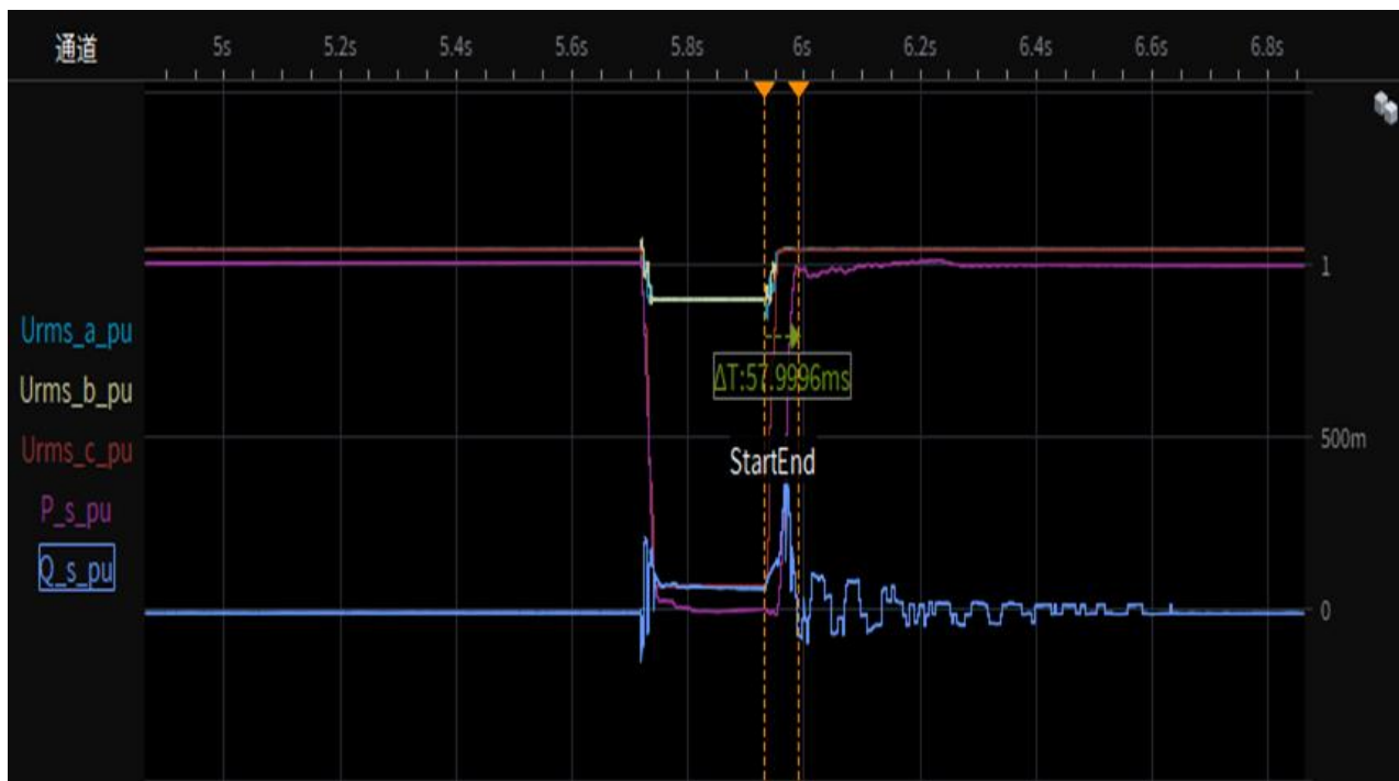
Test 1a-2.4 Depth of fault phase: 0.1p.u., two-phase-asymmetrical (type D), 95% load restoring time
