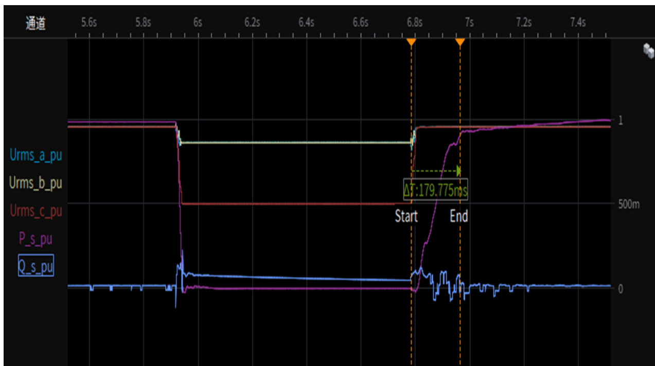
Test 3a-2.4 Depth of fault phase: 0.5p.u.,two-phase-asymmetrical (type D), 95% load restoring time
