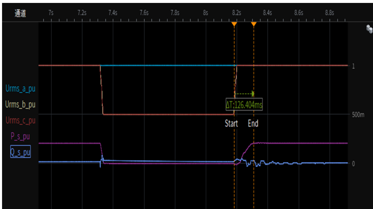
Test 6-1.4 Depth of fault phase: 0.5p.u., LV two-phase-asymmetrical (type D), 20% load restoring time
