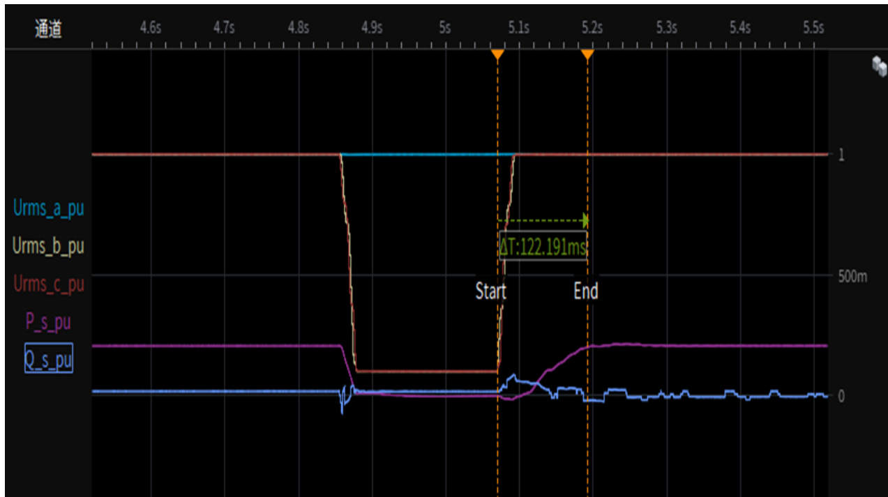
Test 5-2.1 Depth of fault phase: 0.1p.u., LV two-phase-asymmetrical (type D), 95% load Test overview(voltage,current,active and reactive power)
